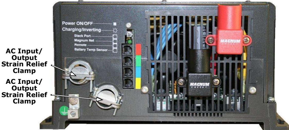
Figure 2-8, RD Series Inverter/Charger - AC Wiring
