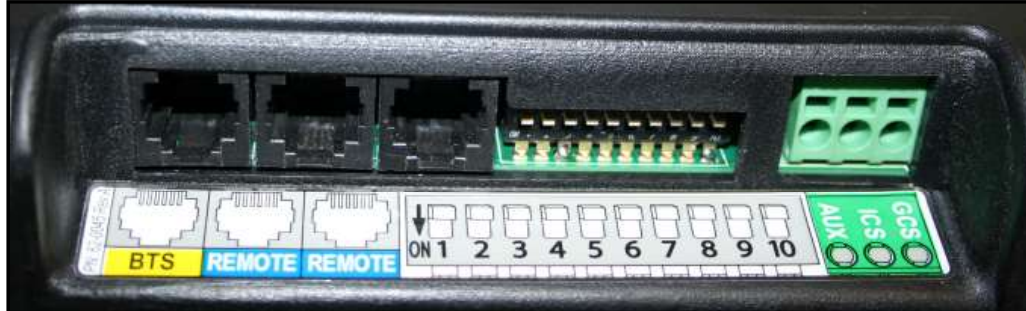
Figure 2-5, MMSA1012's 3-Port Terminal Block
